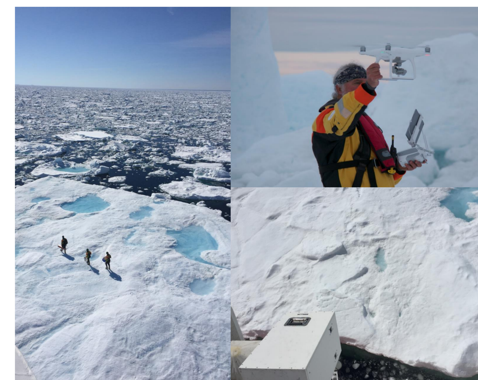
Figure 2. Images of: 1) floe surface sampling, 2) drone image capture and 3) in situ data collection using the PMW radiometer.
