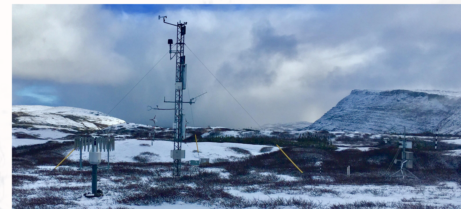
Left: Geonor precipitation measurement Middle: SILVA tower with eddy covariance measurements Right: Tundra station with radiation measurements
