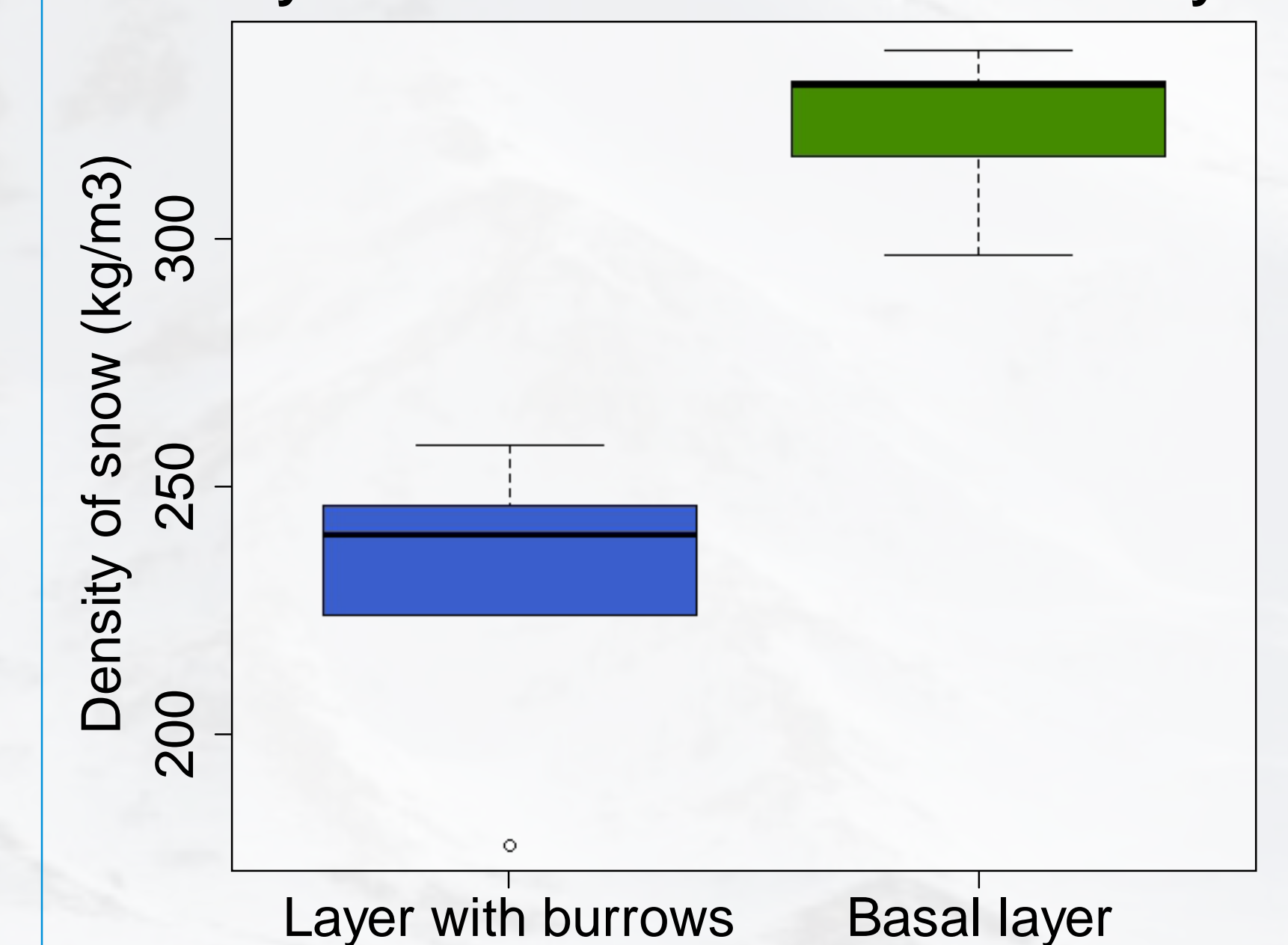
Difference between density of snow layer with burrows and snow basal layer
