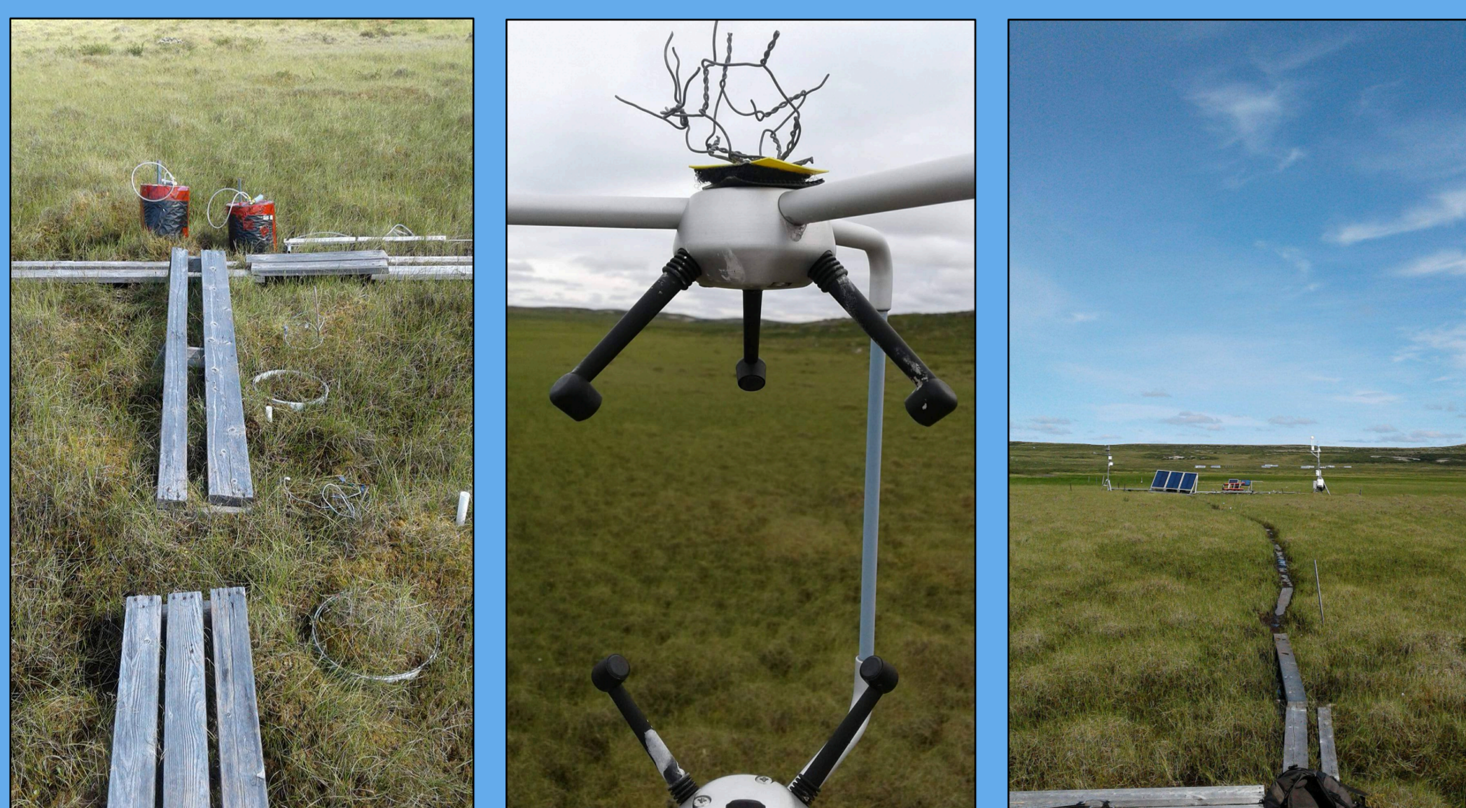
Figure 7. View of 2 of 16 collars where opaque chambers were positioned (left). View from the 3-D sonic anemometer, part of the eddy covariance (EC) instrumentation used to measure 30 minute F_{\text{CH}_4} (middle). Distant view of the EC system including open-path gas analyzers and anemometer (right). Depth to water table (WTD), 0-20 cm volumetric water content (VWC), air and peat temperature were also measured.
