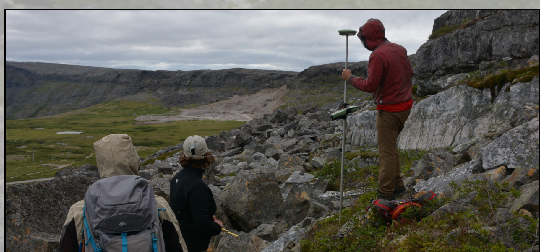
Figure 3: DGPS survey and debris sampling on a talus slope (P. Sæmundsson, 2017).
